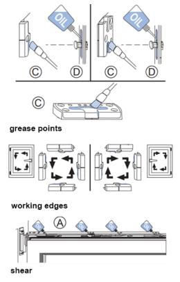
Figure 1 shows possible lubrication points that should be lubricated at least once per year. Points A, C, D = points where lubrication is necessary for the proper functioning of the fitting.
